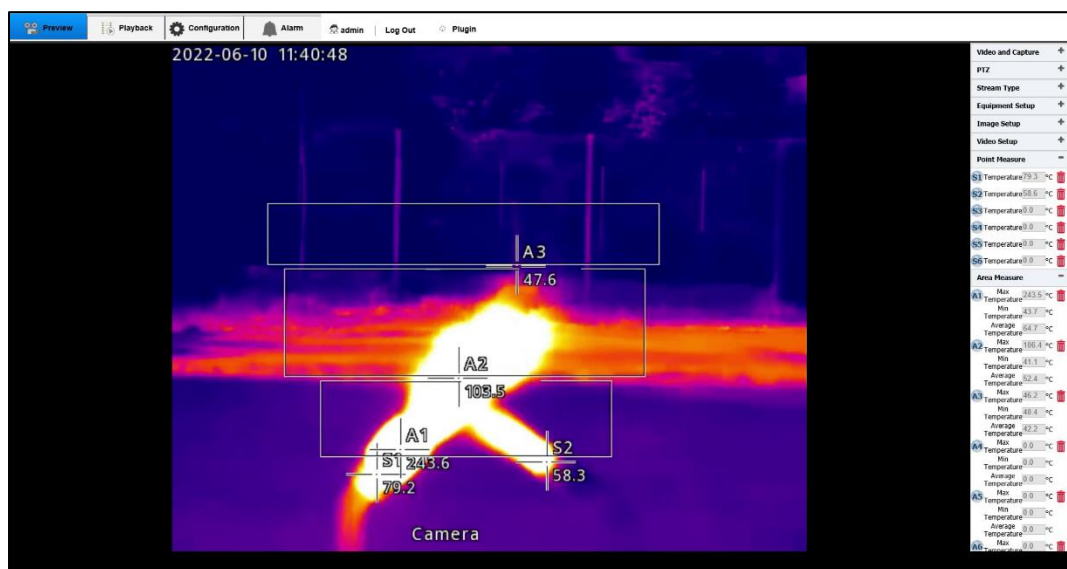
Configurations for Radiometric Temperature Measurement
